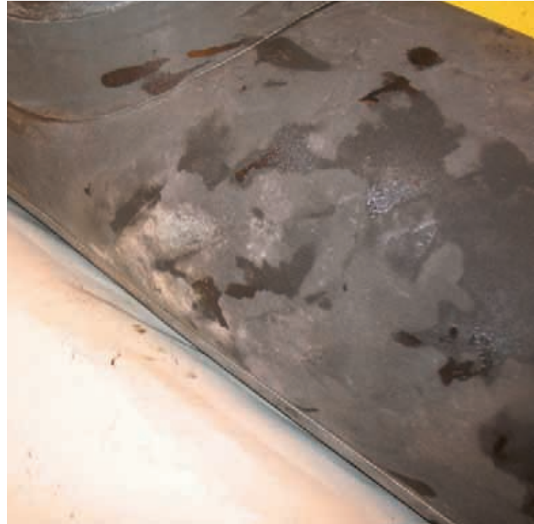
Support frame after incorrect storage
