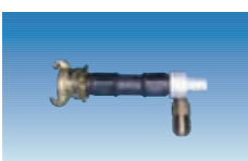
Art.-No. 1700018300 Vacuum adapter for quick deflation of the support frame. Connect snap-coupling onto air supply, pressure should be between 4 and 6 bar (58/87 psi)
